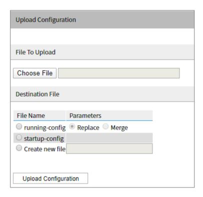
If the target is running-config, the file will be applied to the switch configuration. This can be achieved in two ways:
