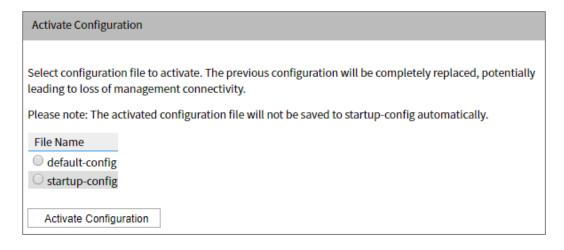
Select the file to activate and click "Activate Configuration". This will initiate the process of completely replacing the existing configuration with that of the selected file.
