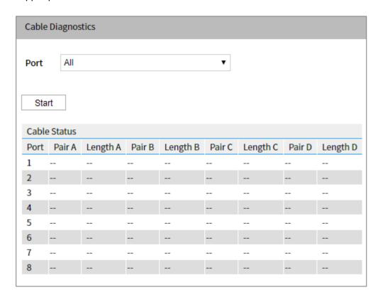
Press "Start" to run diagnostics. This will take approximately 5 seconds. If all ports are selected, this can take approximately 15 seconds. When completed, the page refreshes automatically, and you can view the cable diagnostics results in the cable status table. Please note that VeriPHY is only applicable to cables with a length of 7-140m.
